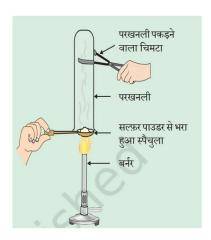
Pratyush took sulphur powder on a spatula and heated it. He collected the gas evolved by inverting a test tube over it, as shown in figure below.
