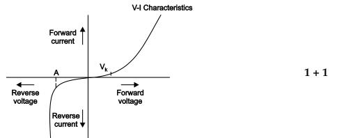
**Breakdown voltage :** It is the reverse voltage at which the breakdown of junction takes place and reverse current increases rapidly. It is shown by the region *OA*. If reverse current increases the safest rated value of diode then it will get damaged.
