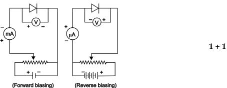
At some forward voltage *i.e.*, 0.7 V for *Si* and 0.3 V for *Ge* known as knee voltage the potential barrier is almost eliminated and the current starts flowing and curve rises sharply as shown in Fig.
