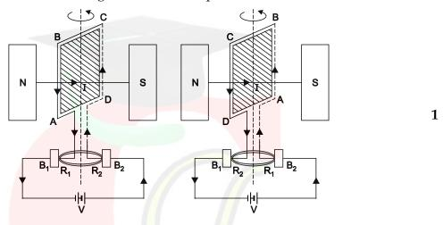
**Working:** As the armature coil is rotated in the mag. field angle  $\theta$  b/w field and normal to the coil changes continuously. An emf is induced in the coil. The direction of induced current is shown in figure.
