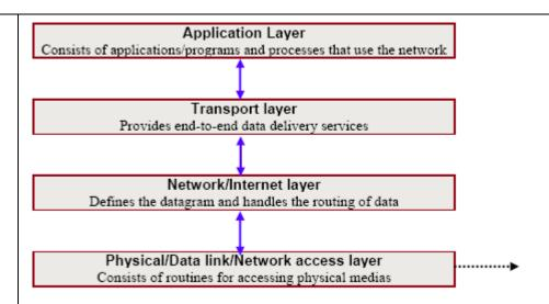
The TCP/IP model serves as a roadmap for effective communication among devices on a network, ensuring a seamless exchange of information. Comprising four layers, each layer performs distinct functions to facilitate efficient communication:
